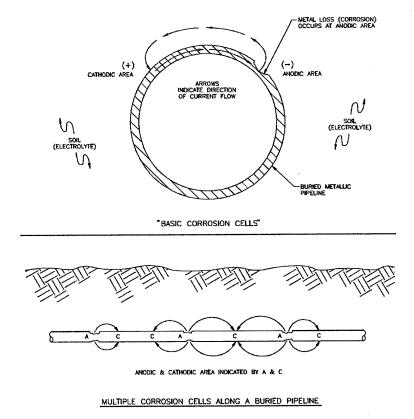
Figure 2 is a diagrammatic presentation of corrosion with conventional current direction shown.
